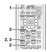
After completing the adjustment, press the TEST TONE button again.
